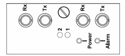
Figure 9: Fiber Serial Interface (ST Connector)
